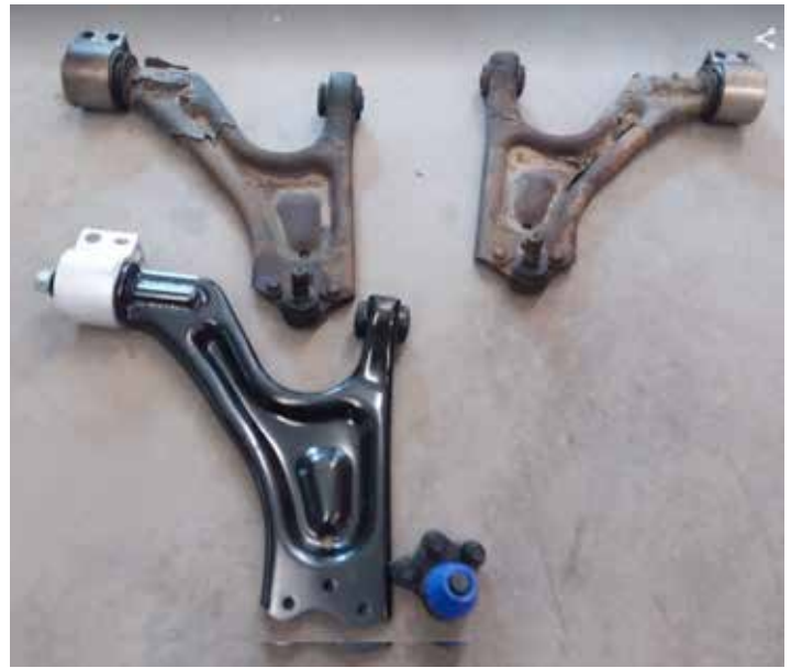
Lower front control arms. Bushings wear out and are hard for DIY to replace but these new control arms have the bushings and a new ball joint and most anyone could install them. Remember, these were done in pairs!
