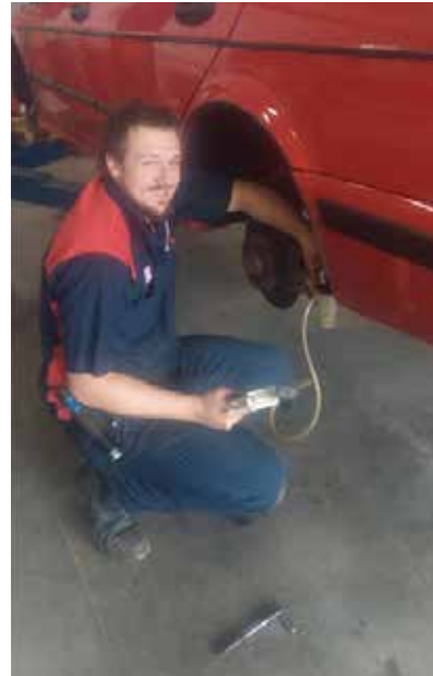
Paul Seline, technician, Saints Automotive using hand suction pump to safely change brake fluid. All photographs provided by the author.
