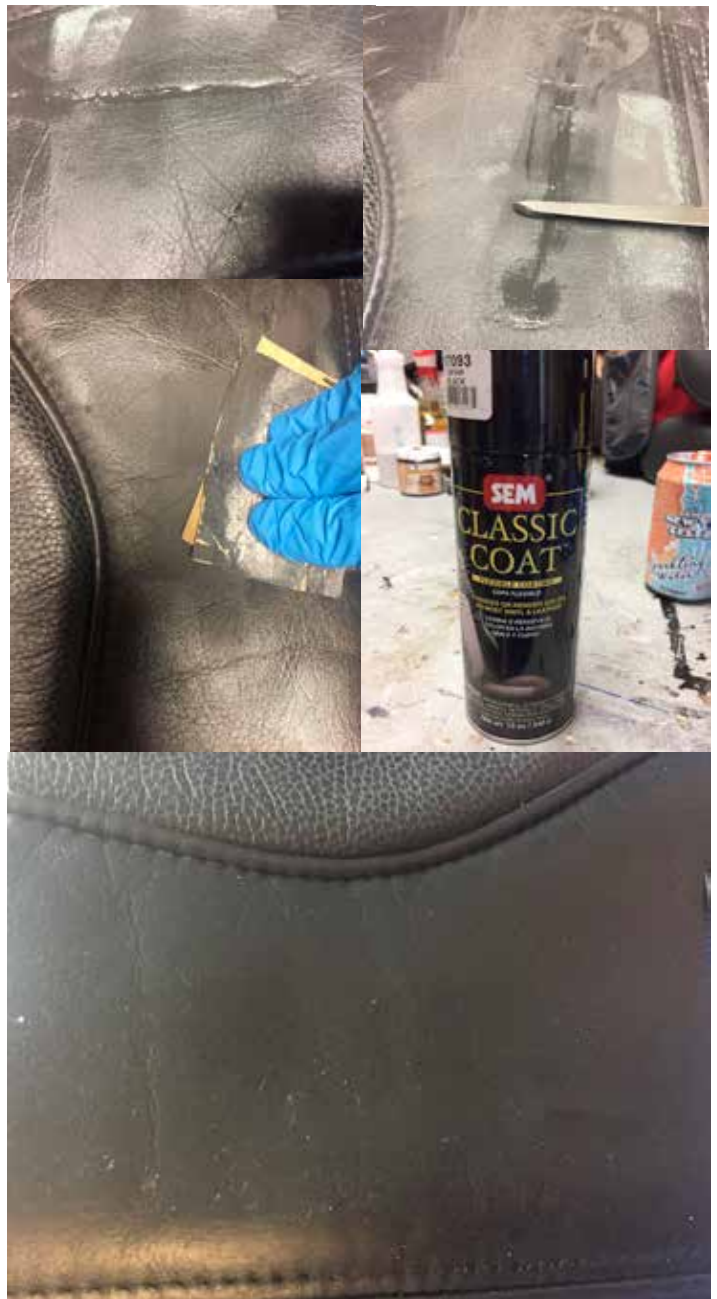
Rip in leather coated with SEM Classic Coat and Acrylic top coat.
