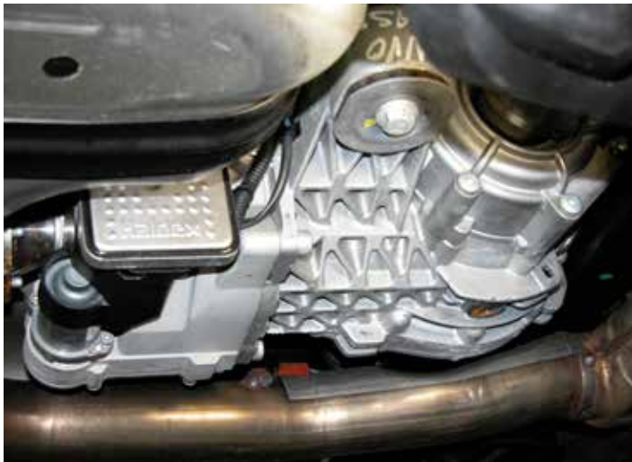
The guts of the Haldex system. Photograph by Seth D. Bengelsdorf.
