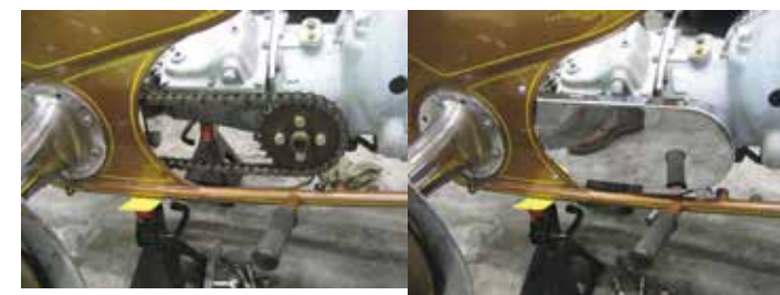
The builder of the trike added gears (left) to modified inner drivers. Chromed covers (right) hide the chains that transfer power back to separate rear axles.
