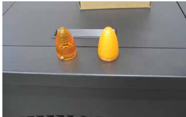
A 3D printer was used to reproduce the turn signal lenses (original on left).
