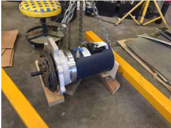
Motor with assembled spacer, adapter and clutch in place. I still needed to make a front motor mount.
