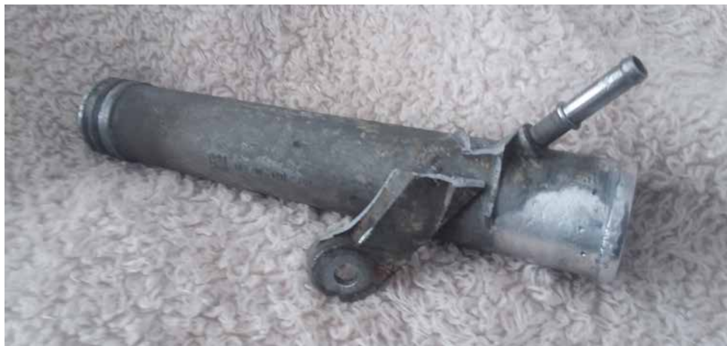
What is it? It is a cast aluminum tube 8 and 3/4 in Long outside diameter at the Left End is 1 3/8 in with two o rings and the right end of the tube is 1 and 5/8 inch outside diameter and you can see the bracket that's broken off. Photograph by the author.
