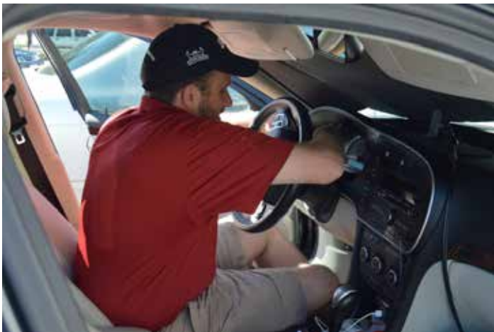
Pop the old air bag out. Careful with the connections! Plug and replace. Jonathan Diagnault of Viking Automotive shows how it's done! Photographs by the author.
