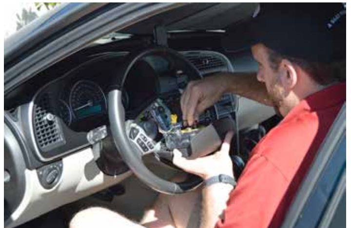
Pop the old air bag out. Careful with the connections! Plug and replace. Jonathan Diagnault of Viking Automotive shows how it's done! Photographs by the author.
