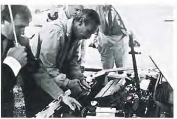
Sealing Power-train components with plumb-bobs.
