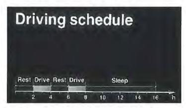
The driving schedule drawn up for the test consisted of 2 hours of driving followed by a rest period of 2 hours, thereafter a further 2 hours of driving and 2 hours of rest. After an 8 hour rest (sleep) period the schedule was repeated three times. After 3 full driving schedules, equaling 40 hours, drivers then had 16 hours free to relax.
