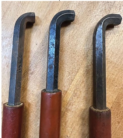
Wrench needed to remove the full Level plug on side of transmission. Picked these up at a flea market.
