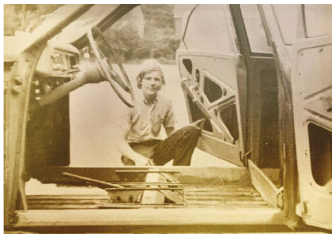
Bill patching the floor pans in a 1957 model 93 that his Dad gave to him when he was 14.
